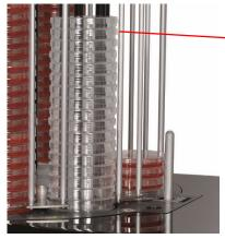
If the lid outer diameter (at bottom) is too large, the lid gets stuck between the carousel rods.
