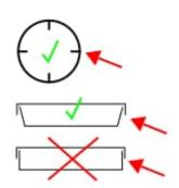
Use dishes with ventilation camps on the inside of the dish lid. Ventilation cams prevent the formation vacuum, the base can fall down.
