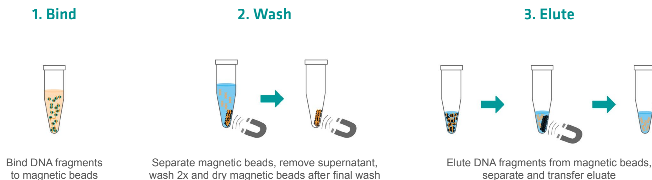
Figure 1: Step-by-step procedure of the MAGFLO PCR purification protocol.
