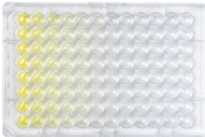
Figure 5: 2-fold serial dilution of tartrazine in a 96 well flat-bottom plate.
