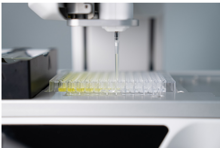
Figure 4: The ASSIST PLUS and VOYAGER performing serial dilution of tartrazine.
