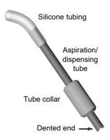
The aspiration/dispensing tubes delivered with the DOSE IT facilitate the dosing process and are fitted on the end of the tubing. The aspiration tube is dented on one end in order to guarantee a free flowing of the liquid entering the tubing. Make sure not to insert the dented end of the aspiration tube into the silicone tubing.
