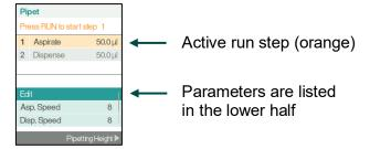
Insert the GRIPTIPS into the liquid to be transferred. Press and release **RUN** to aspirate the volume selected in the first step.
