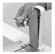
To access the laser insert a tool into the round hole and lever out the silver cover of the tip detection sensor housing. The cover is held in its position by magnets and pulls off with little force.
