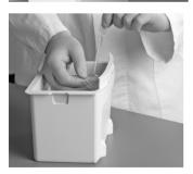
Place the **sensor reflector**  $(\underline{8})$  on the waste bin.
