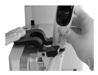
To release the pipette lift the black gripper by pushing down the left end.
