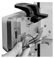
To adapt the holder for an 8- or 16 channel VIAFLO pipette fold both silver levers (a, b) down as shown beside.
