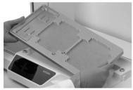
Hold the **deck**  $(\underline{7})$  with both hands and place it over the corresponding positioning studs. Press down firmly until you hear a click.
