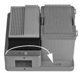
Attach the second stage to lift the 12.5 or 125  $\mu l$  tip rack so that both racks are the same height when using 300  $\mu l$  LONG or 1250  $\mu l$  GRIPTIPS.
